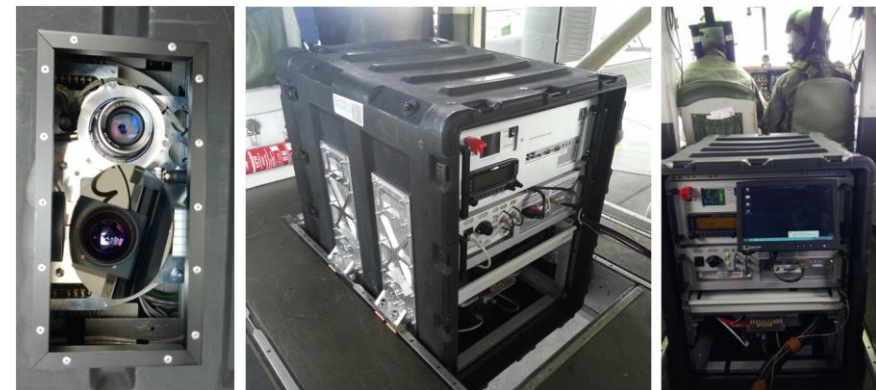
Figure 2. Components of the airborne segment at a Pilatus Porter PC6 AA
