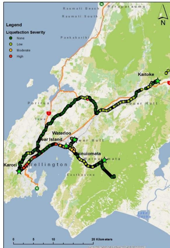
**Figure 3 Wellington water supply mains, with soil liquefaction potential. Stars represent water sources.**
