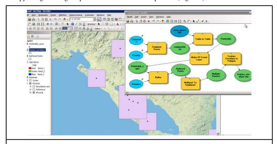
Figure 1. The ASAP tool shown in the ArcGIS. ASAP is based on a custom model built using the ArcGIS model builder tool (shown on the top right of Figure 1). Text-based disaster descriptions are inputted into the model and processed into area of interest (AOI) polygons. In this example, a disaster description from Nicaragua has just been processed resulting in four AOI polygons (shown
