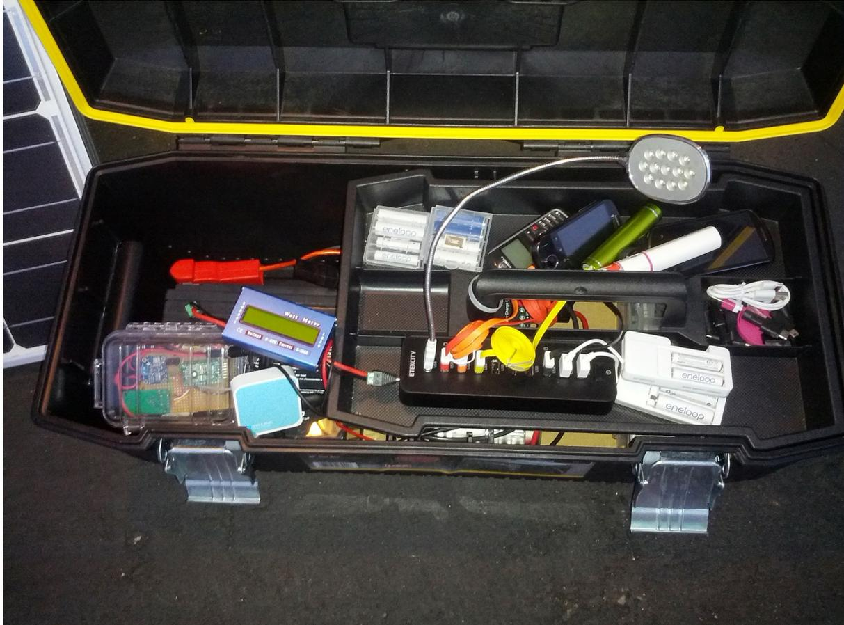
**Figure 1.** A reference charging kiosk, containing current and voltage sensing and control equipment (left), tray with 10 port USB hub, LED light, phones, batteries, and flashlights (right), battery, charge controller and power distribution unit (below other items), and 100W solar panel (background).
