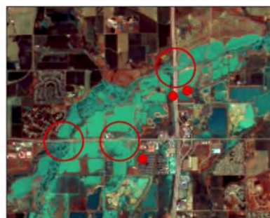
Figure 6. Flooded bridges over I-25 Highway shown on the Landsat 8 image as large circles. Overlaid geo-tagged tweets shown as small filled circles.
