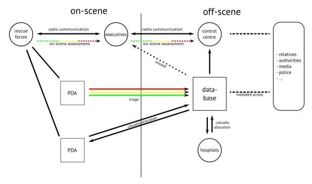
Figure 8. The integration of the SOGRO-IS in the MCI response network.
