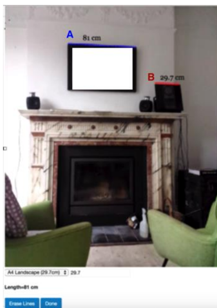
Figure 3. The interface to measure objects: a line is drawn on the known object (red line (B) known length 29.7); a second line (A) is drawn on the target object: the system displays the length (81 cm).
