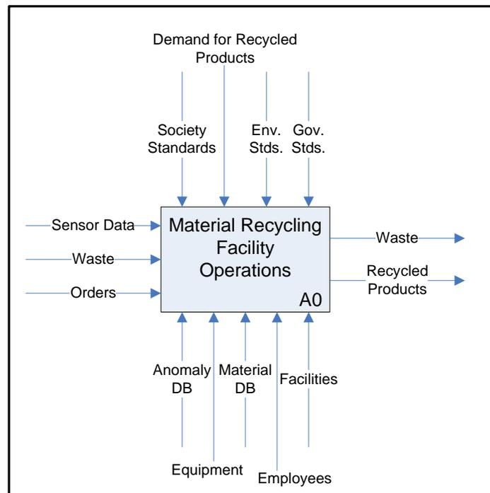
Figure 4. High-level IDEF0 View of the MRF
