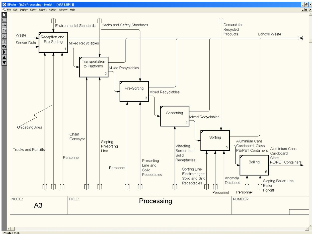
Figure 5. Third level IDEF0 model of the Processing activity.
