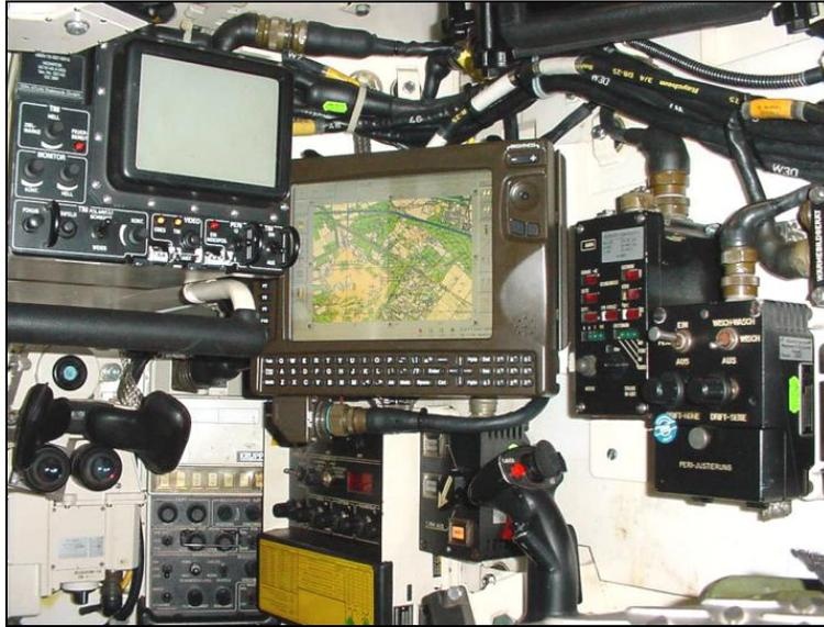
**Figure 3. BMS workstation installed in Leopard tank.**
