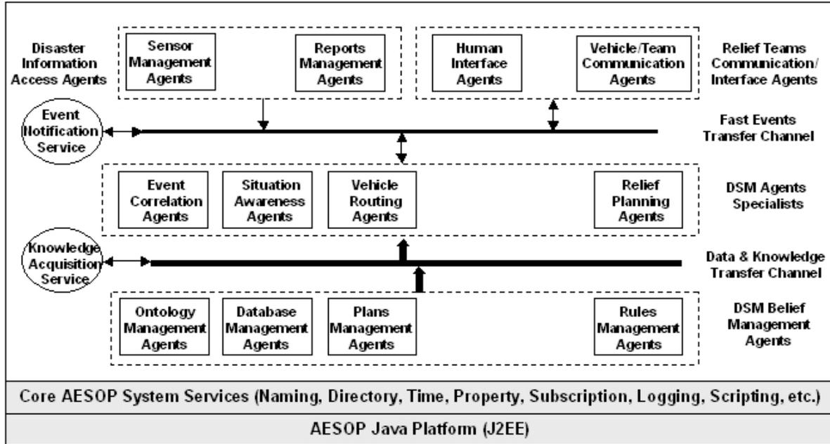
Figure 7. Distributed AESOP Platform for DSM
