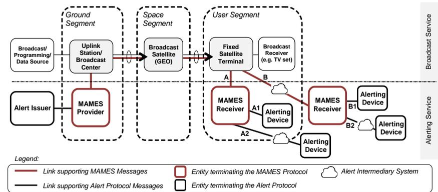
**Figure 3: MAMES integration into a broadcast fixed satellite system**
