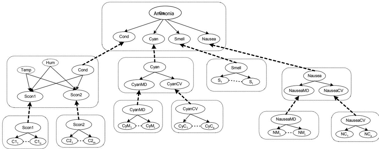
**Figure 1.** A DPN fusion organization where each dotted rectangle represents a DPN agent. Thick dashed lines represent communication between cooperating agents, which share partial fusion results. Each agent makes use of a local Bayesian Network, a probabilistic model that captures specific expertise over a certain domain. The agents assemble their local models into a distributed causal model that supports evaluation of the hypothesis about the existence of “Ammonia”.
