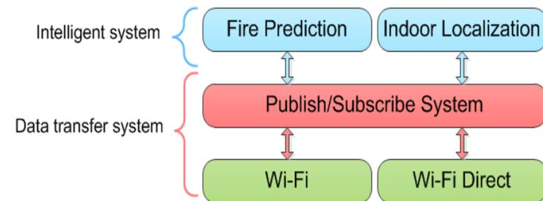
Figure 1: Overall Architecture of SmartRescue
