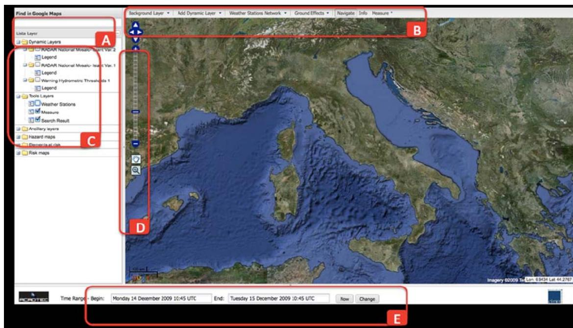
**Figure 1** Dewetra has five control areas, which define the main functionalities of the system (see A, B , C , D, E in the figure). A - the Google Maps® engine; B - the main upper toolbar contains the groups of information layers and the functionalities available; C - the navigation tree containing dynamic and static layer; D - a set of navigation tools; E - time range and scales for the representation of data.
