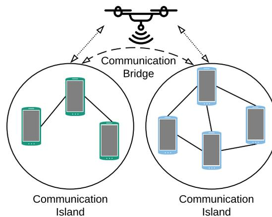
**Figure 3.** Communication amongst intermittent communication islands in a DTN-MANET requires nodes to act as communication bridges. UAVs are either acting as message relays by positioning themselves in communication range between two near islands, or by providing more efficient means of physical message transport between remote islands due to their mobility.
