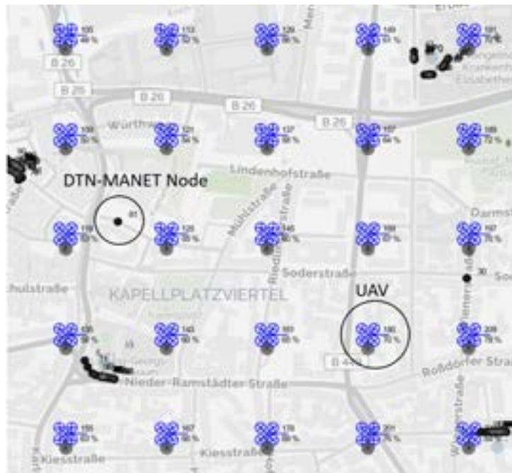
**Figure 6.** UAVs form a relay mesh in an urban environment. The graphical representation of SIMONSTRATOR.KOM shows UAVs hovering above the map and DTN-MANET nodes on the ground. Nodes use pedestrian walkways when moving or gather around important locations. UAVs are visualized with their current battery levels.
