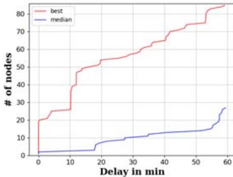
**Figure 2.** Number of reached nodes and the corresponding propagation delay during the field test. Messages had a lifetime of 60 minutes (Álvarez et al. 2018).
