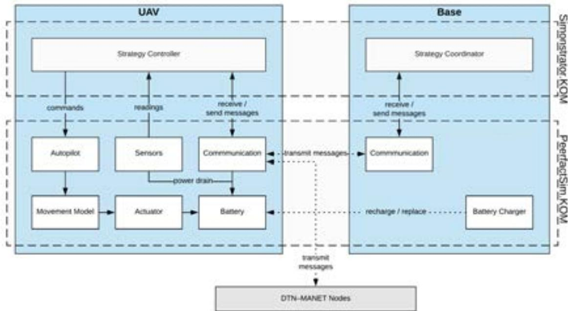
**Figure 4. Overview of system components for UAVs and base stations comprising the UAS in the simulation platform, with their respective location in SIMONSTRATOR.KOM and PEERFACTSIM.KOM architecture. Dependencies between components are indicated by lines and arrows, dotted lines show non-permanent connections like message transfer over the network or during the battery recharging process.**
