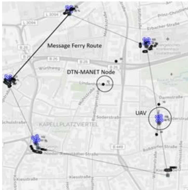
**Figure 7. Message ferry UAVs move between five communication islands. They hover above each location while exchanging messages with the DTN-MANET nodes on the ground, before moving to the next. UAVs only visit statically defined islands, thus, nodes out of transmission range cannot be reached.**
