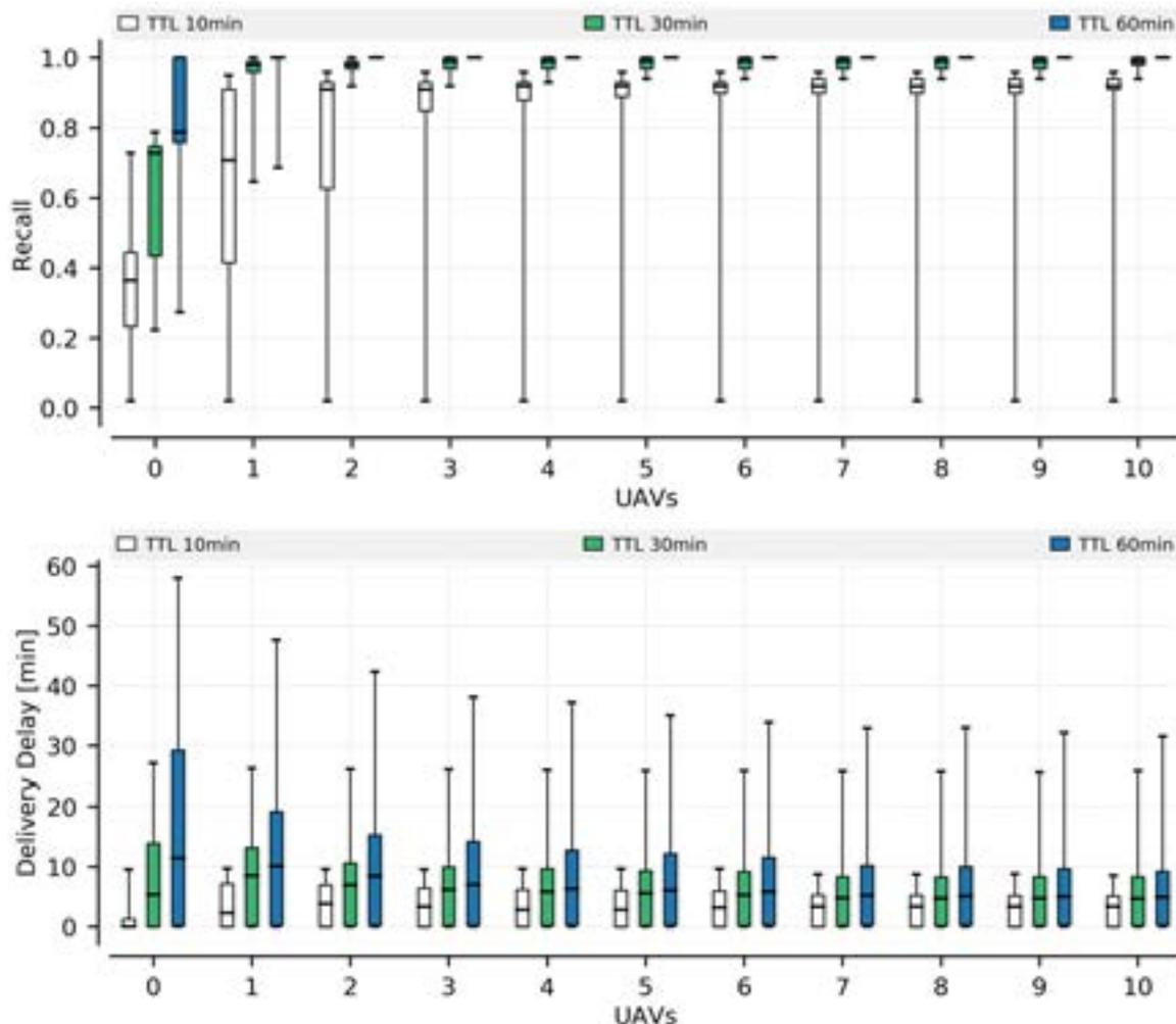
**Figure 10. Recall and delivery delay variance shown for increasing numbers of UAVs. The TTL was set to 10, 30 and 60 minutes, respectively. As indicated, a few UAVs already significantly increase the communication performance, especially with longer TTL. The setting '0 UAVs' shows the unsupported DTN-MANET performance.**
