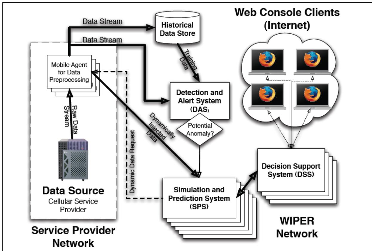
Figure 1: An overview of the prototype WIPER system.
