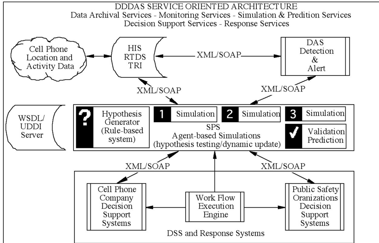
Figure 2: The proposed Service Oriented Architecture of the WIPER system.
