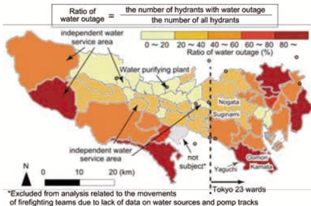
Figure 8. Average ratio of water outage and location of water purifying plant
