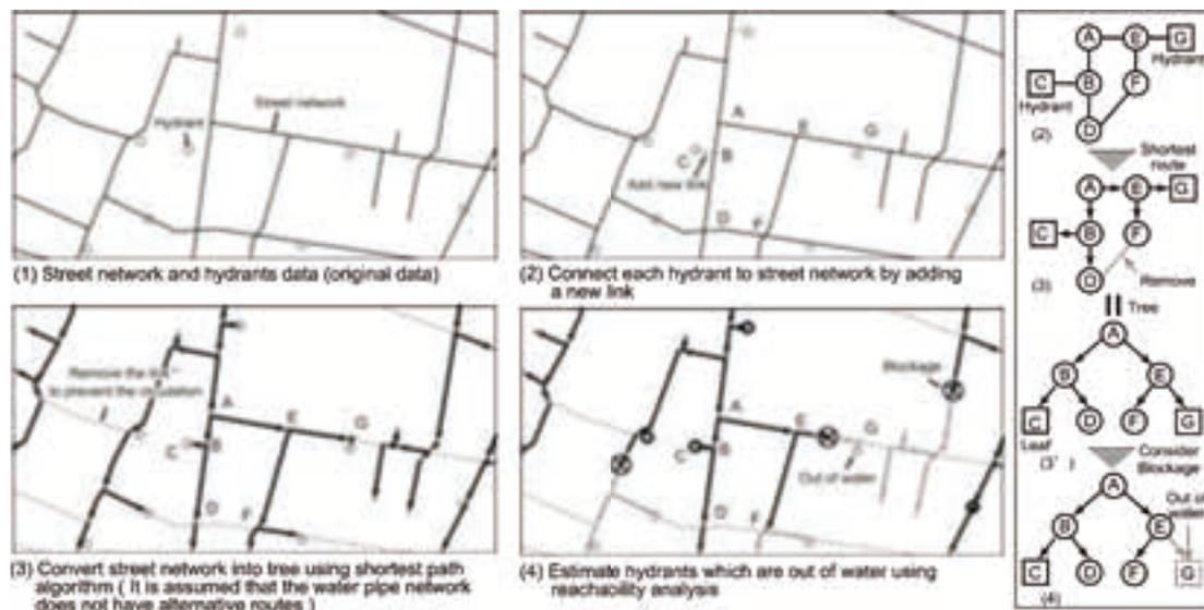
Figure 1. Construction of water pipe network and estimation of water outage
