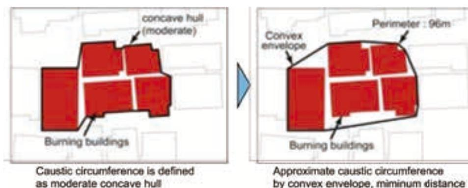
Figure 4. Approximate caustic circumference based on fire-spread simulation
