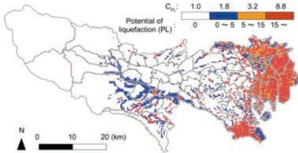
Figure 2. Potential of liquefaction (PL) in Tokyo Metropolitan area
