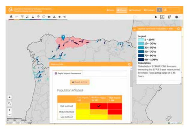
Figure 2. Screenshot of EFAS web interface with the layers identifying areas where there is high probability of floods in the following 48 hours and rapid impact assessment
