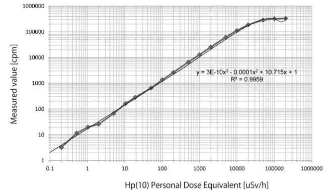
**Figure 4 Measurement range for Cs<sup>137</sup> (Kuipers et al., 2011)**
