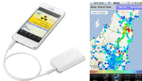
Figure 1 Pocket Geiger Device and software
