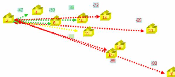
Figure 4. Signal strength view from Node 2.
