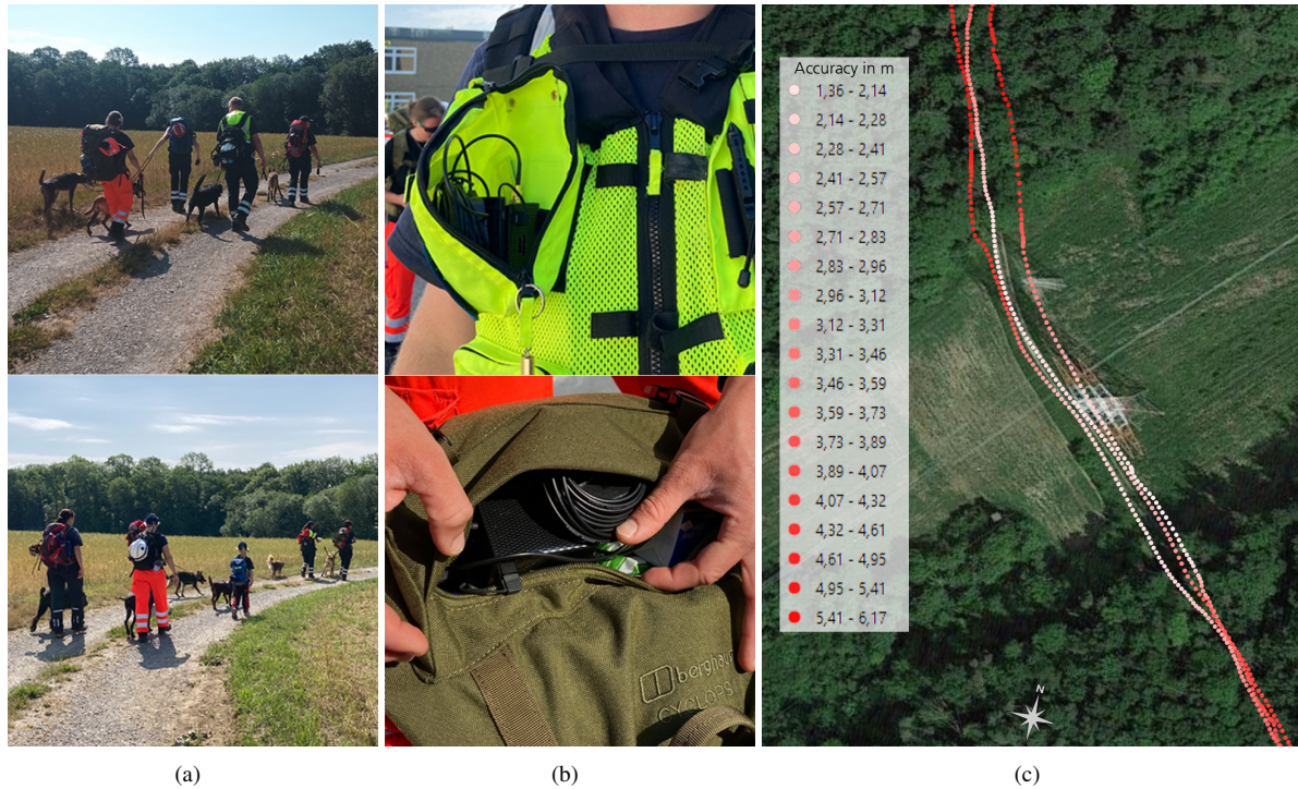
Figure 3. Tool usage and performance in Mosbach: two rescue dog squads (a), Tool positions (b) and GNSS accuracy changes when entering or leaving the woods (c).
