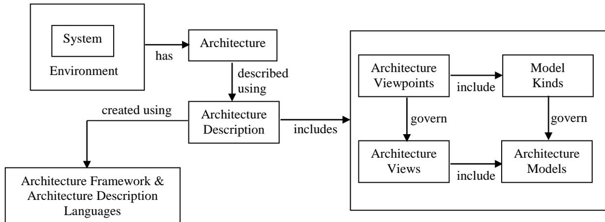
Figure 3. Meta-model of architecture concepts used for CMI CF design, after ISO/IEC/IEEE 42010
