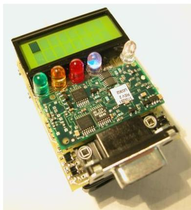
Figure 4. Electronic triage tag with colour LED technology. Photo see Gao et al 2007: 207.
