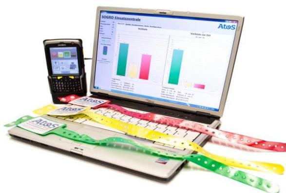
Figure 5. SOGRO 2012: digital triage system with PDA and colour-coded RFID tags. The PDA transmits the triage status to a data centre from where it can be accessed.
