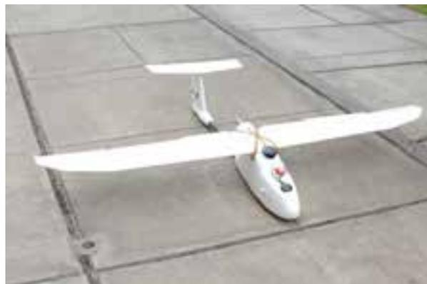
Figure 4. 1880 - Skywalker UAV model for multipurpose appliances
