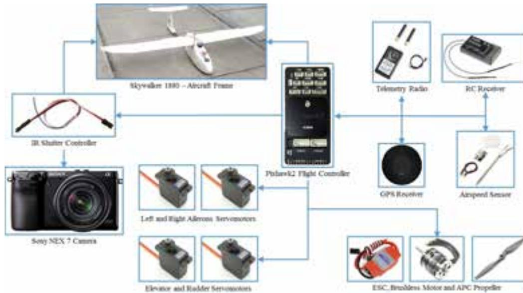
Figure 5. An overview of the fixed-wing UAV proposed system
