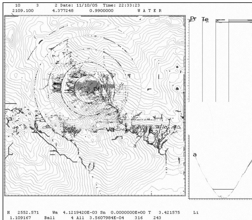
**Figure 3. Scenario of debris-flows activation in the epicenter of earthquake with earth surface distorts and soil resistance reduces, where: on the bottom – current data for the Virtual Gauge (VG): H-Elevation, Wa -Water depth, T-Air Temperature, Li –Soil resistance, Ball - power of earthquake, All – Sediment thickness. Other signs are the same as on Figure 2.**
