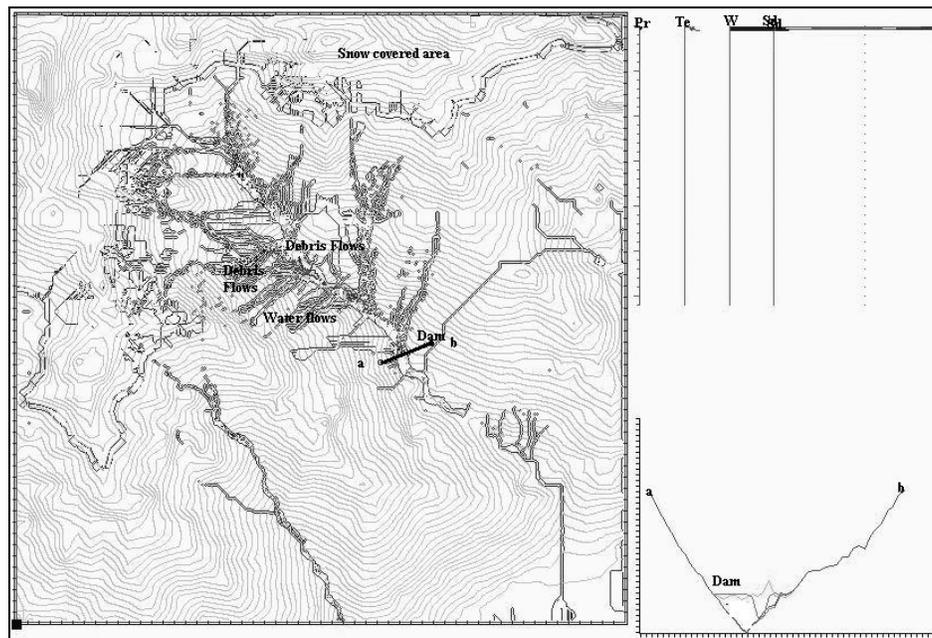
**Figure 2. Scenario (with a 10m resolution) for activation of erosion and debris-flows after local storm upstream, where: Precipitation (Pr), Temperature (Te), computed Water discharge (Wt) and Sediment Discharge (Sd), 'Virtual' Dam (a-b), which being cut by debris-flows.**
