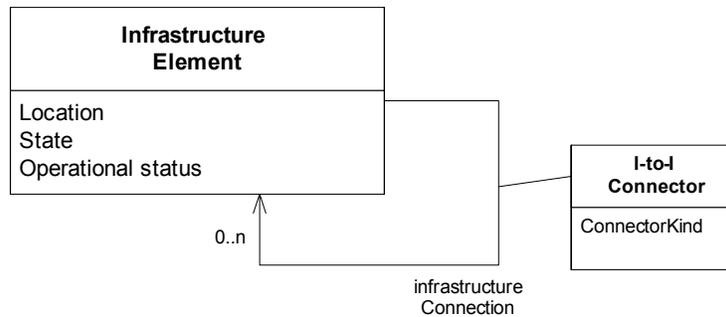
Figure 8: Physical connection between 2 different infrastructures (class diagram)
