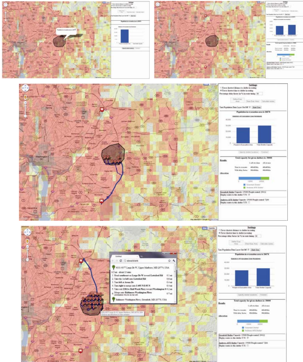
Figure 1: The current EvacSpace prototype allows users to create an evacuation area, specify shelter locations, and identify possible routes to those shelter locations along with estimated driving times.
