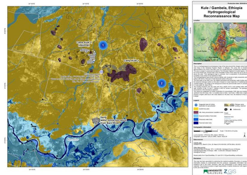
**Figure 4: Example for a hydrogeological reconnaissance map in a sedimentary environment, using Landsat and SRTM data. Areas threatened by flooding, which are unfavourable locations for wells, are mapped blue.**
