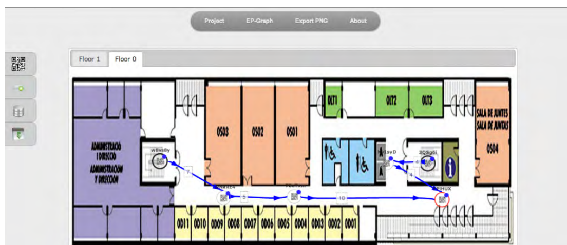
Figure 2. Screenshot of the Building component: graph representation of the evacuation routes
