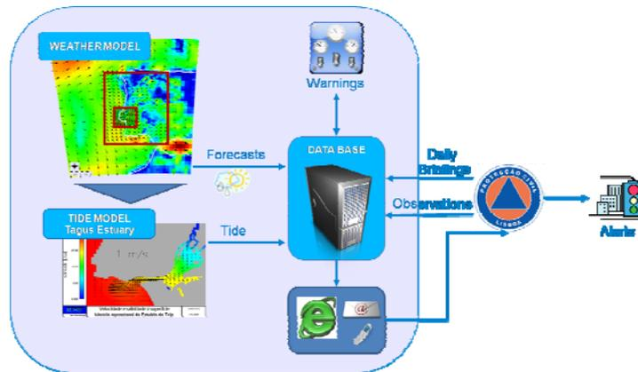
**Figure 1. Architecture of the Integrated Operational System for Meteorological Risk in Lisbon Municipality (OS).**
