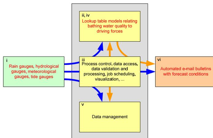
**Figure 2. Elements of a water quality forecasting system to forecast bathing water quality**
