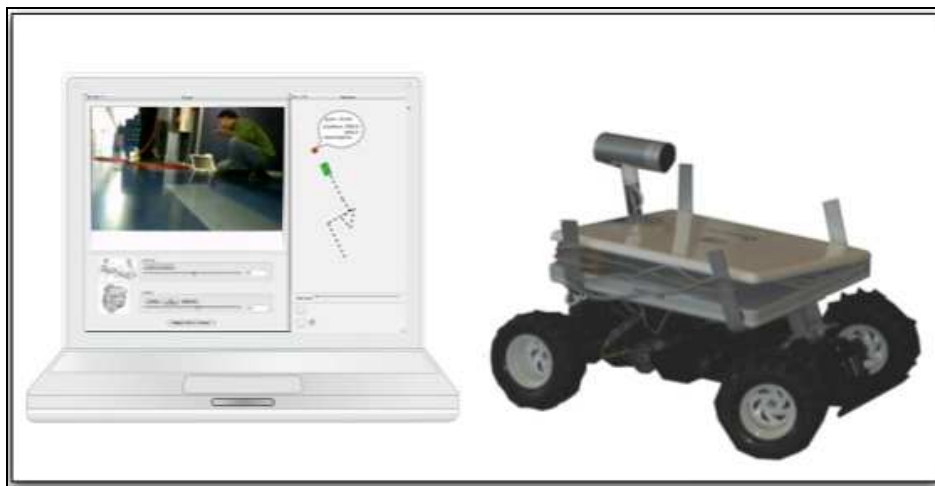
Figure 3. The robotic sensor platform dubbed iRescue can be controlled either wirelessly or tethered by any machine running the iSearch control software. In this case, the control software is utilizing a live video sensor feed along with a dynamic shared map representation.
