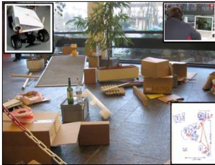
Figure 5. In the simulated search and rescue task, the robot operator communicates with an off-site navigator over an early version of the iSearch software to jointly build a map of the environment while exploring the disaster area for victims.
